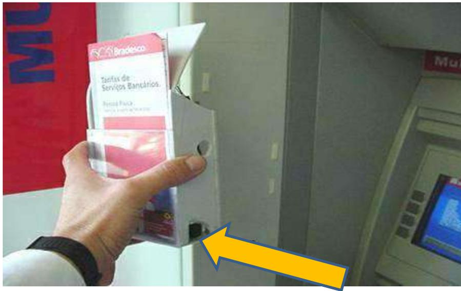
Take a closer look at the **brochure holder** –a **pin-hole** Camera has been installed. This is done to capture images of the keypad and customers inputting their PIN.
