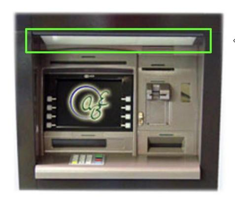
Photo shows a PIN capturing device fitted to the top of the ATM. These devices are usually difficult detect.
