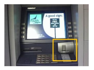
Skimmer device attached to card entry slot.
